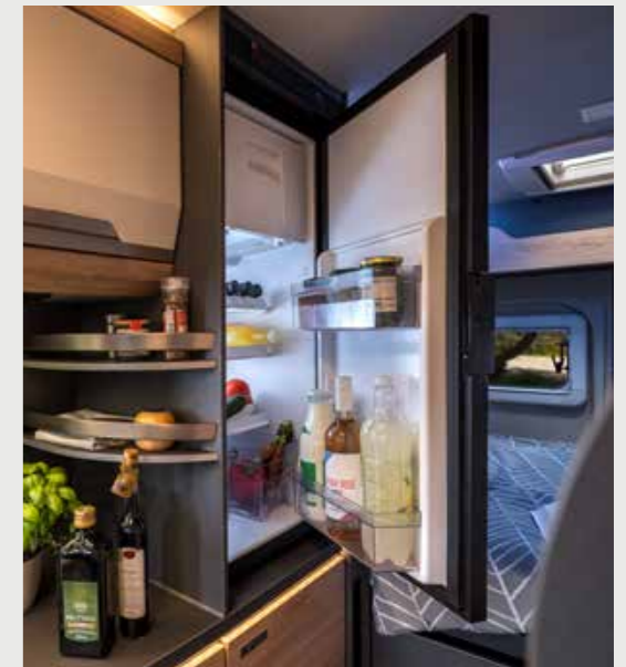
BOXLIFE PRO 600 STREET. With its 90 litre capacity and 7.5 litre freezer compartment, the compressor refrigerator in the BOXLIFE PRO provides plenty of space.
