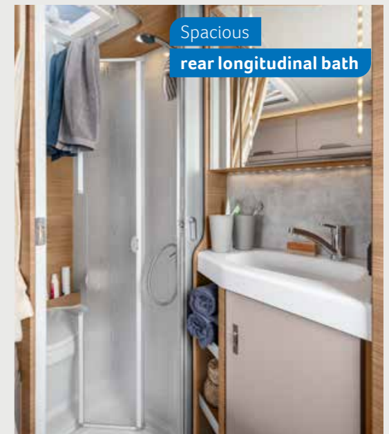
VAN TI 650 MEG. A clever swing wall in the comfort bath ensures that you quickly have an extra generously sized shower cubicle. A smart magnetic closure simply seals the shower door watertight.
