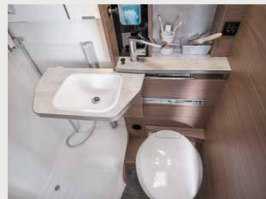
TOURER VAN 500 MQ. The washbasin can easily be moved to the side, so the toilet can be used at any time – even when the shower is folded out.
